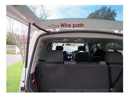
The reverse light signal can be tapped behind this panel. You have to remove the rear light cluster, the rear light wire at the connector is the wire furthest on the right (use a multimeter to confirm) - you have to unwrap the cloth tape and tap the wire further down (once inside the cab, past the rubber boot)
