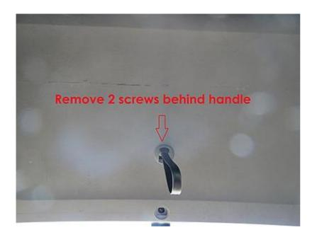
Then the entire back panel of the boot just unclips. Start by pulling at the far end (I put my finger in the emergency boot release hole and yanked away.)
