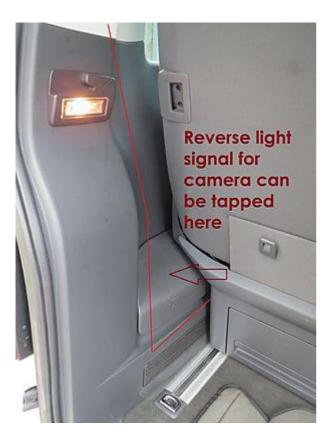
Push the wire along here behind the trim. Make sure it doesn't foul the back seat. This took a bit of fiddling to get the wire right by pulling and pushing.
