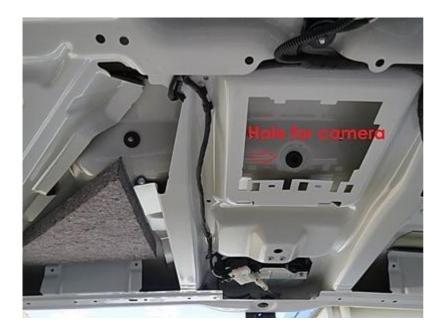
Run the wire along here. Silicone spray really helped get the wire through the rubber tube.
