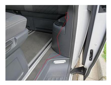
You can unclip the entire step by pulling straight up but putting it back on is a total b!tch.
